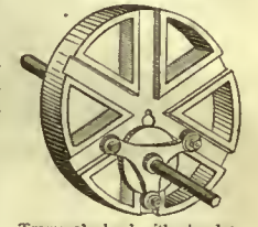
Trammel-wheel with six slots.
